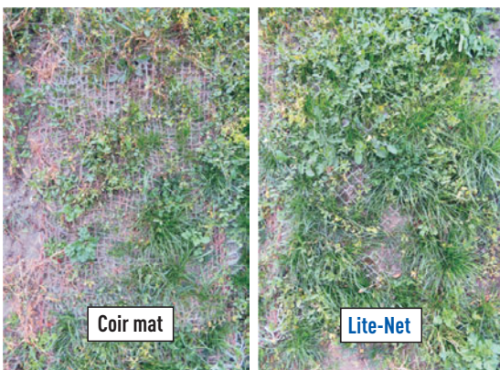
Investigations BOKU Vienna: Vegetation coir mat (left) and Lite-Net (right) after 3 months of extreme drought
