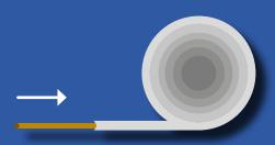
Unroll the LITE-NET with a slope at the edge of the roof, and install the protected irrigation pipe: Once slightly raised at the edge of the roof, and then with a distance of 50-60 cm between each section in the further roof area.
