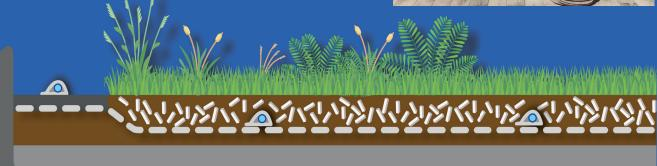
Alternatively, you can fix the nonwoven-covered irrigation tubes superficially on or in a layer of gravel. Disadvantages: UV attack, mechanical damage. Advantages: Easy control and replaceability.
