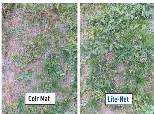
Vegetation on coir mat (left) and LITE-NET (right) after 3 months of extreme drought
